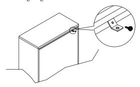
Attach a bracket securely to the back top rail of the furniture using short screw provided, through the smaller hole.
