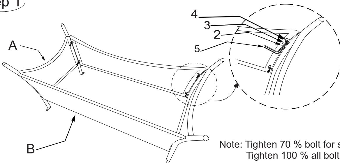
Note: Tighten 70 % bolt for step 1
