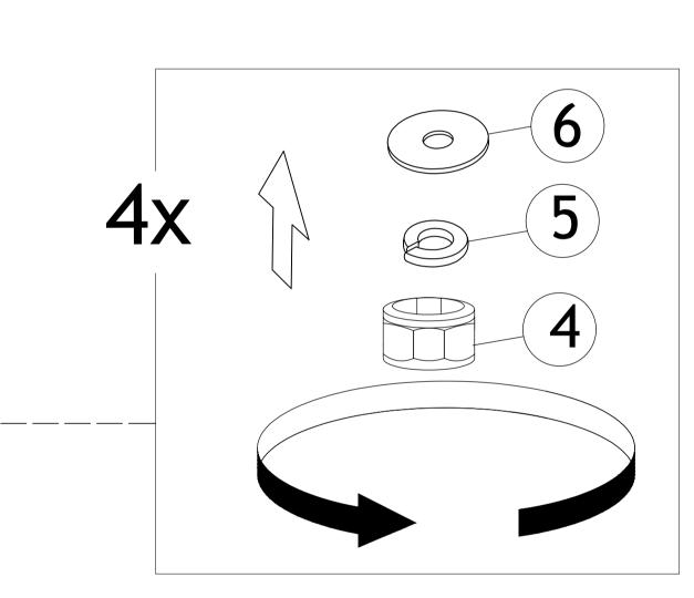
Do not tighten the Hex Nut set completely!
