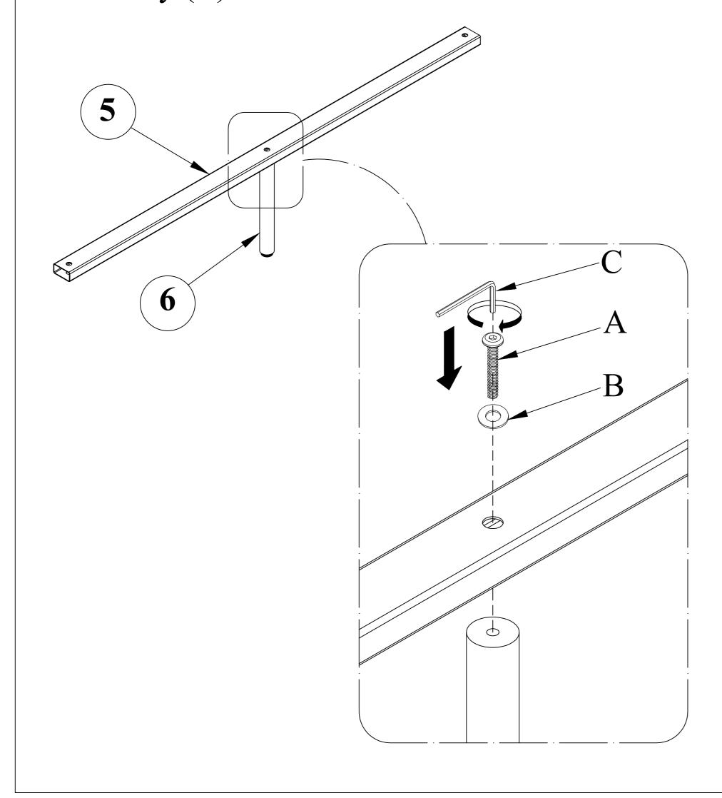
Step 4: Assemble the Slat (5) to the Side Rail (4) by using Allen Bolt (A), Flat Washer (B) and
