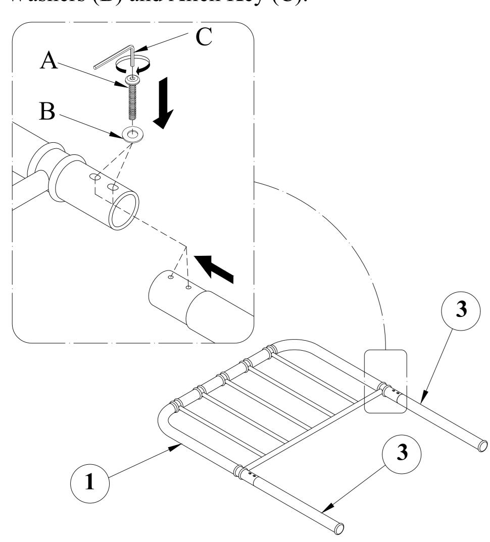
Step 2: Attach the Side Rails (4) to Headboard (1) and Footboard (2) by using Allen Bolts (A), Flat Washers (B) and Allen Key (C).
