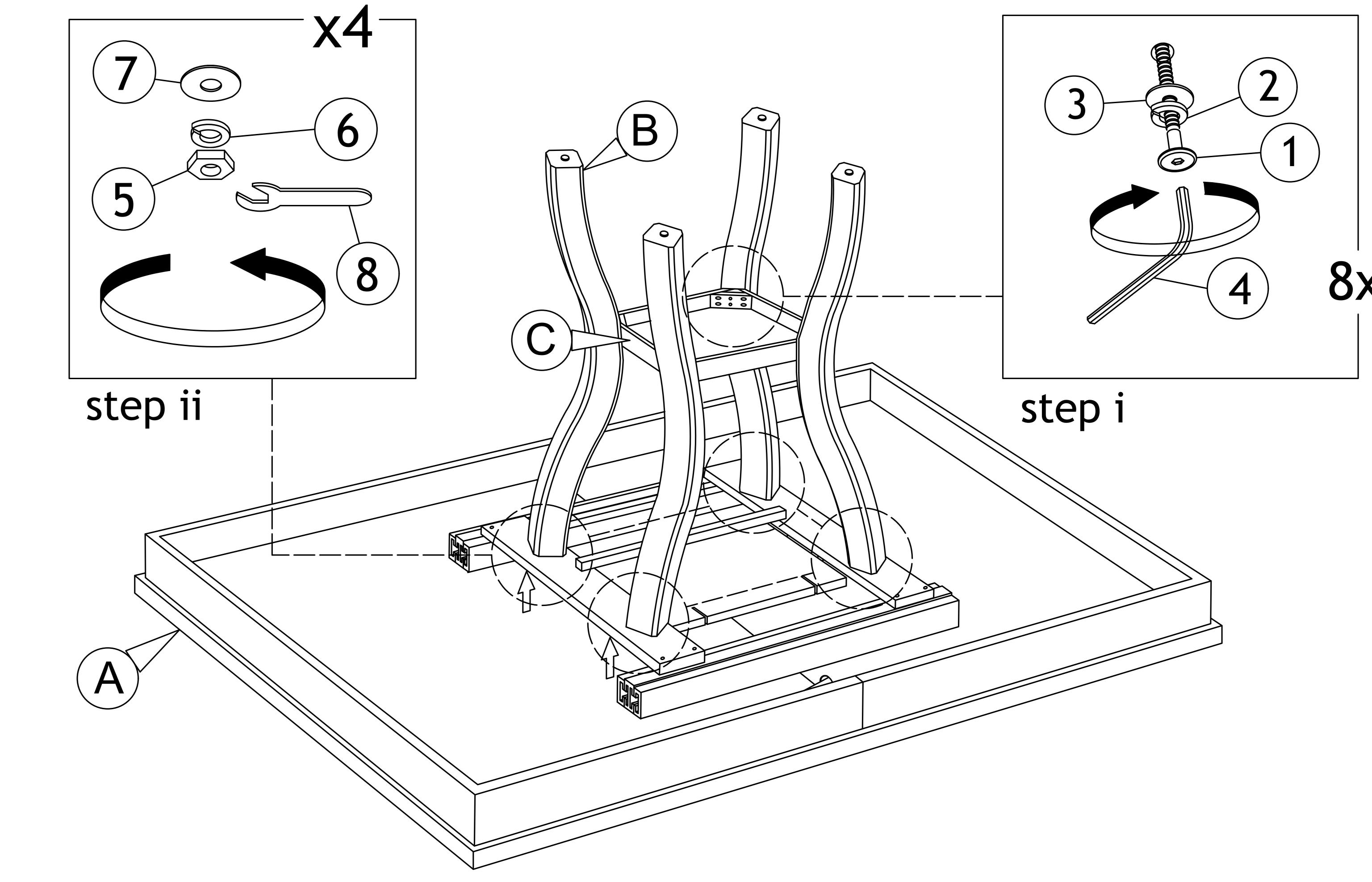
step i : tighten part (A) with part (B) first.
