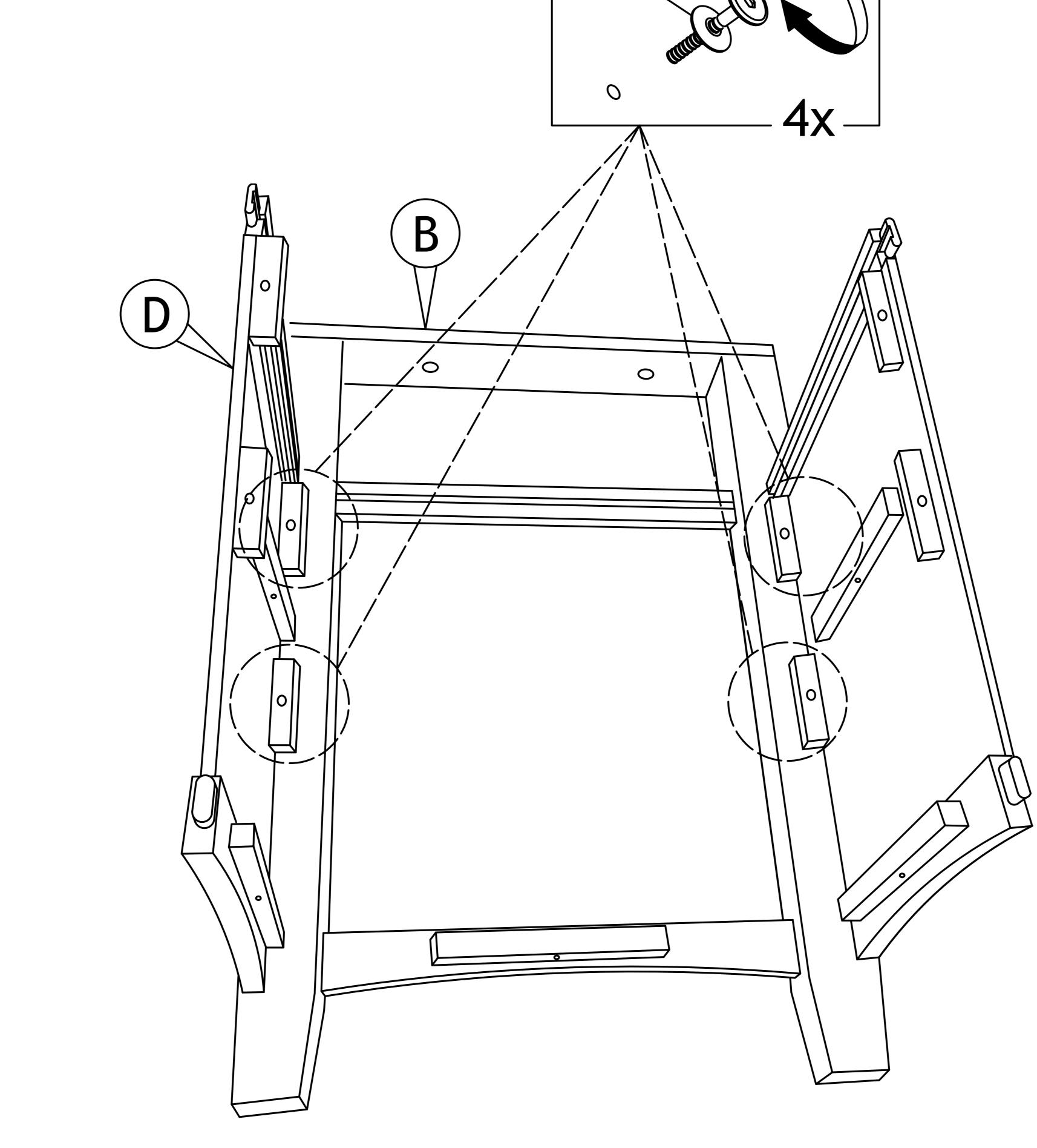
Attach part (D) with part (B). Do not Tighten any hardware completely!
