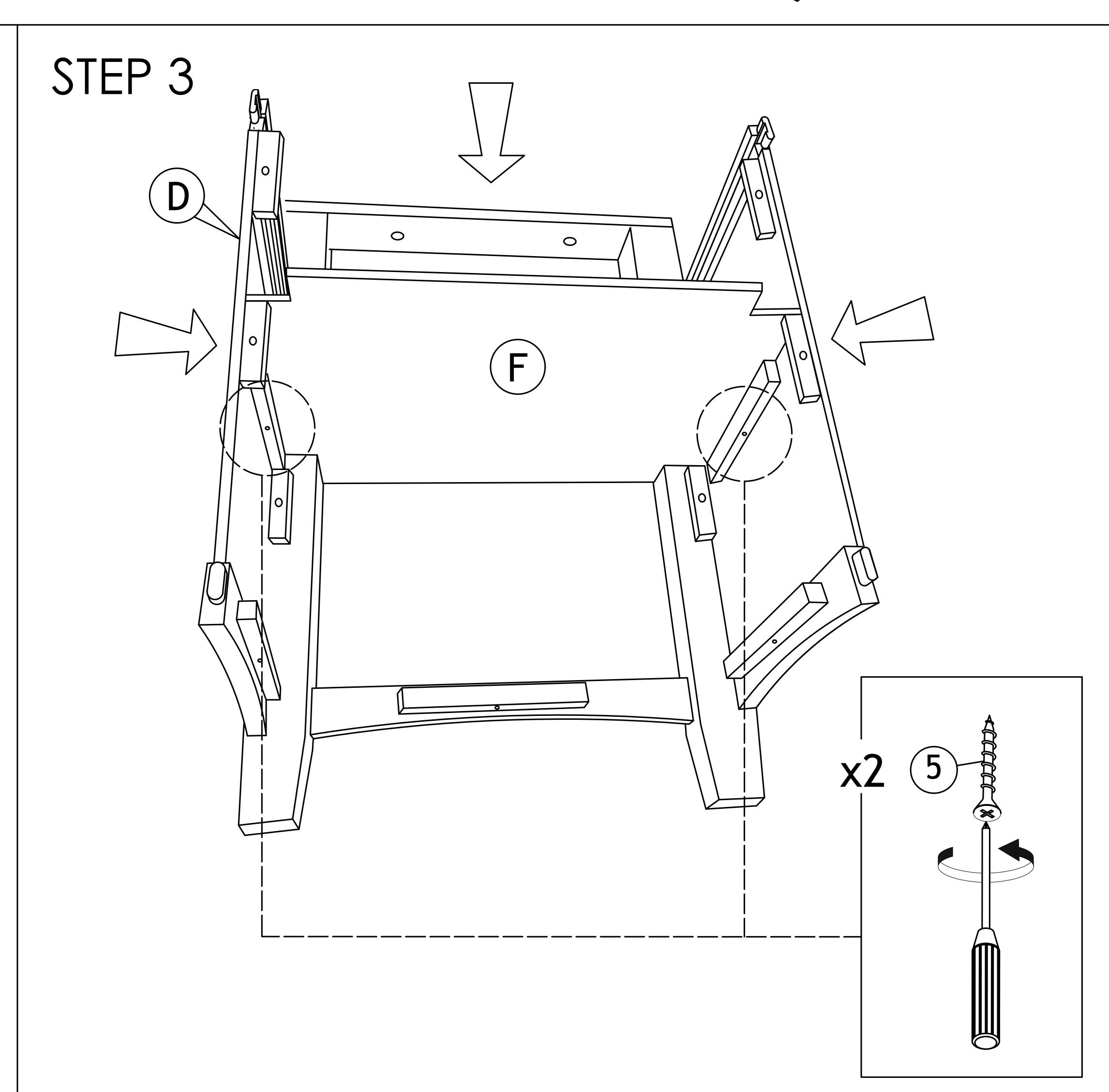
Insert Panel (F) and do alignment to fit panel (D) with panel (F) first, then tighten part(F) completely using 2 pcs CSK screw.
