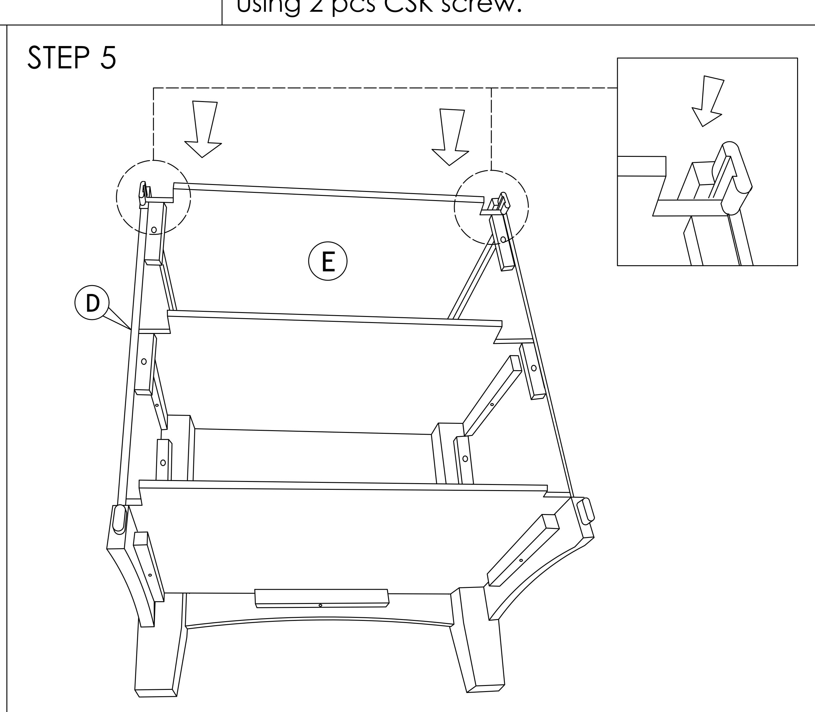
Insert panel (E) through side curve of top of panel (D).
